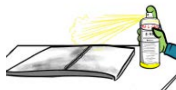
R-503 used as a pre-cleaner spray directly on test surface and wipe clean.
