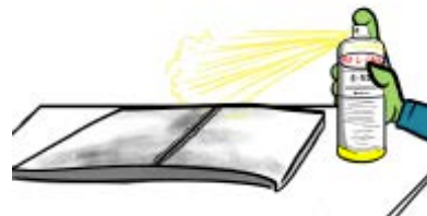
E-59A used as a pre-cleaner spray directly on test surface and wipe clean.
